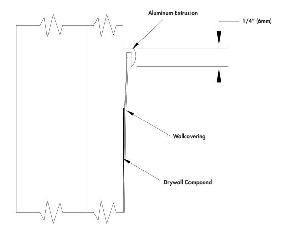
Mechanically fasten with self-tapping drywall screws and/or adhere aluminum extrusion with construction adhesive or contact cement.
