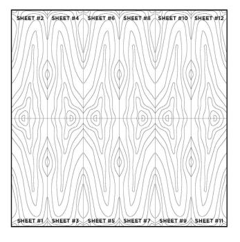
With end matching the sheet on top will be reversed I80 degrees. For example, the top of sheet (#I) will end match to the top of sheet (#2).
