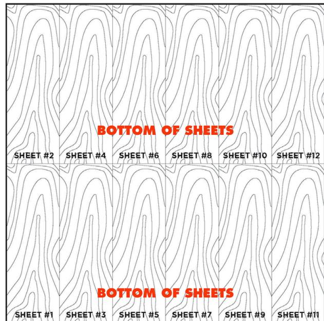
**\*Note:** For best visual of grain pattern, we suggest laying out the sheets prior to installation to determine what direction the sheets go as sometimes "bottoms up" appears more aesthetically pleasing than "tops up". Please confirm with specifier or end user for approval prior to installation.
