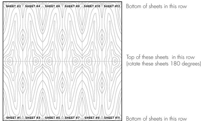
With end matching the sheet on top will be reversed 180 degrees. For example, the top of sheet (#1) will end match to the top of sheet (#2).
