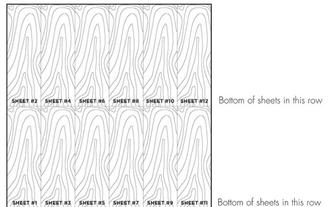
**\*Note:** For best visual of grain pattern, we suggest laying out the sheets prior to installation to determine what direction the sheets go as sometimes "bottoms up" appears more aesthetically pleasing than "tops up". Please confirm with specifier or end user for approval prior to installation.
