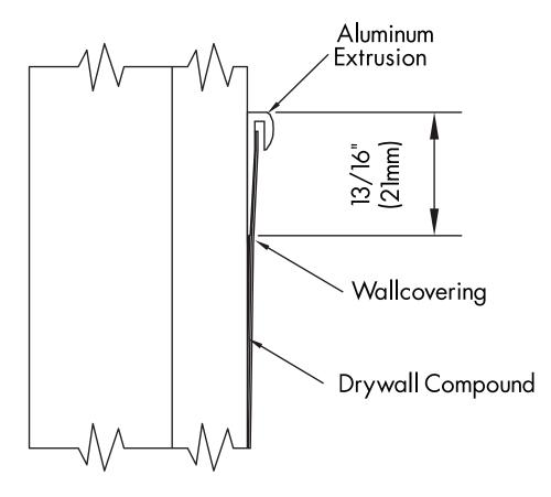
Mechanically fasten with self-tapping drywall screws and/or adhere aluminum extrusion with construction adhesive or contact cement.
