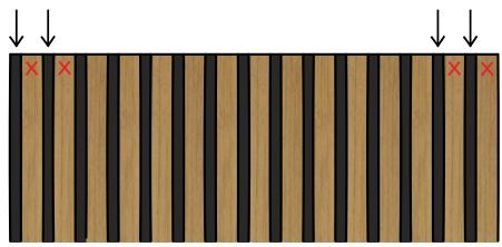
Use the premade shiplap joint to maintain even spacing and to avoid visible seams.
