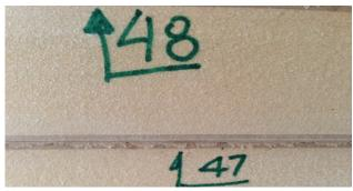
**8.** Mark the bottom edge of the door with sequence numbers so as to insure correct matching on the job site.
