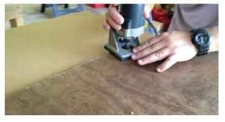
**4.** Using a high speed router, trim the excess veneer from the edges of the substrate.
