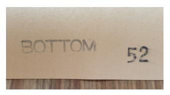
**2.** Locate the Sequence # (in this case 52) and insure that the face you are about to bond is the correct face for the elevation you are working on. Be certain that the sheet is oriented correctly.
