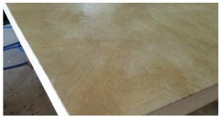
**4.** Spray, roller or brush contact adhesive evenly across the appropriate face of the door core. Insure that you cover 100% of each surface and leave to dry.
