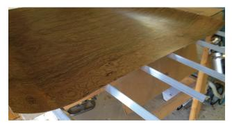
**2.** Place separator sticks on the substrate and then lay the veneer on the separator sticks taking care to insure the glued surfaces do not touch.
