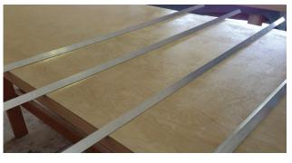
**5.** Place separator sticks on the substrate and then lay the veneer on the separator sticks taking care to insure the glued surfaces do not touch.
