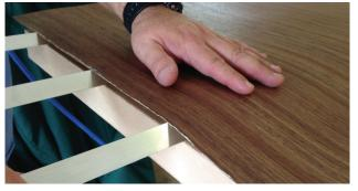
**6.** Remove the separator sticks one by one and smooth out the veneer working from the center outwards. Insure the veneer is pressed firmly down using a straight edge and any air expelled.
