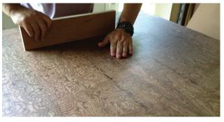
**3.** Remove the separator sticks one by one and smooth out the veneer working from the center outwards. Insure the veneer is pressed firmly down and any air expelled.
