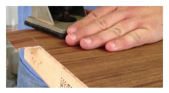
**7.** Using a high speed router, trim the excess veneer from the edges of the substrate.
