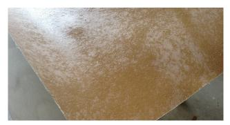
**3.** Spray, roller or brush contact adhesive evenly across the back surface of the veneer. Insure that you cover 100% of each surface and leave to dry.
