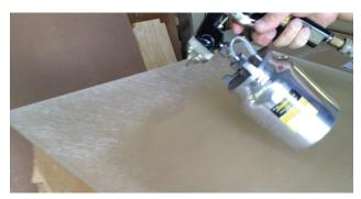
1. Spray, roller or brush 3M-4693H adhesive evenly across the two surfaces to be bonded together. Insure that you cover 100% of each surface and leave to dry.
