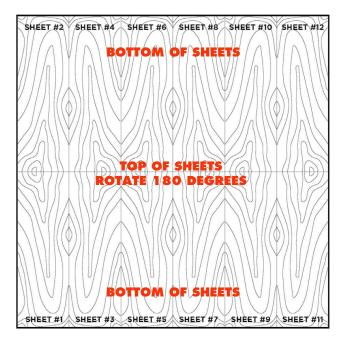
With end matching the sheet on top will be reversed 180 degrees. For example, the top of sheet (#1) will end match to the top of sheet (#2).
